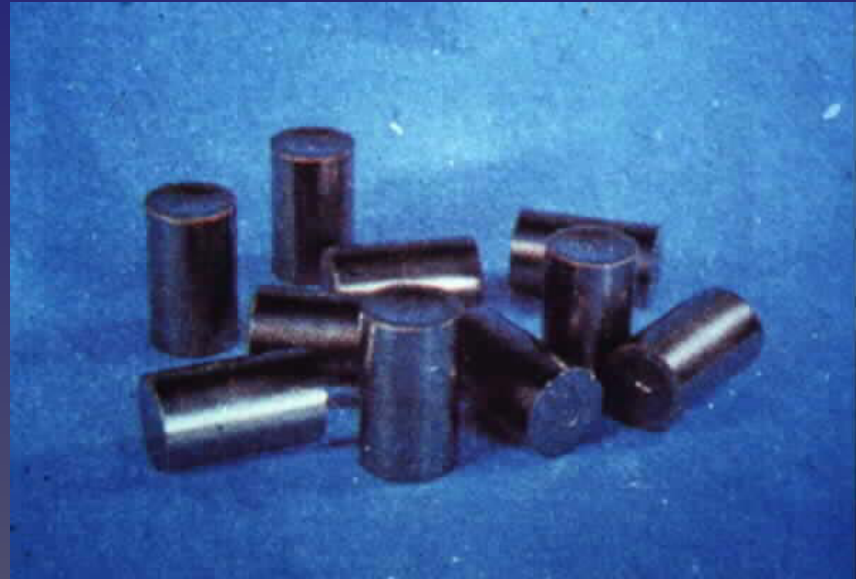
Uranium fuel pellets with concentrated ^{235}\text{U}
